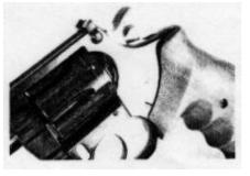
Only one visible seam shows on the frame of the Korth. just below the windage adjustment screw on the left side. The mottled appearance is oil on the frame.
